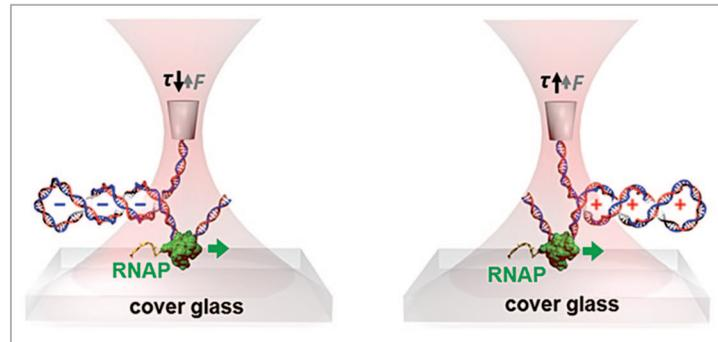
**Figure 1.** Experimental configurations of transcription under torsion using an angular optical trap. RNA polymerase transcribes against either an upstream (-) DNA supercoiling (left) or downstream (+) DNA supercoiling (right). Artwork by Robert A Forties.
